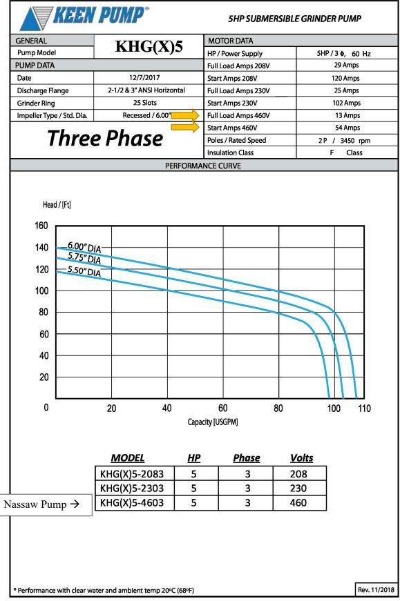
Nassaw Lift Station Pump Data: Keen KHG(X)5-4603, 460V/3Phs.
